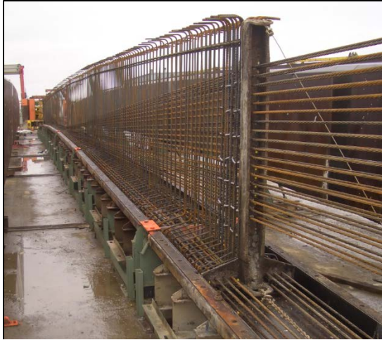
Figure 12: Form Profile with Cage & Strands
